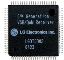
The 5th generation VSB(Vestigial Side Band)/QAM receiving chip
