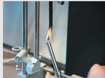
Vertical/horizontal fire test
