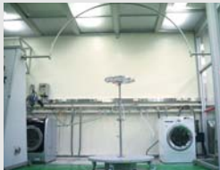
Moisture resistance lab Testing for moisture resistance, fire hazard, arc detection, and electric shock
